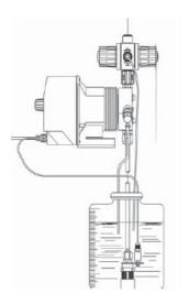
The EMEC Multifunction MF valves which are available either to mount directly to pump or can be wall mounted, combine a pressure relief valve and a back-pressure valve.
