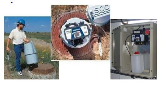
Isco 6712 Sampler. A multi-bottle portable sampler with highly intelligent and versatile programming functionality. It has a built in logger and can be provided with optional plug-in flow modules. It used extensively wherever multi-bottle sampling is required and is also our standard hire sampler.
