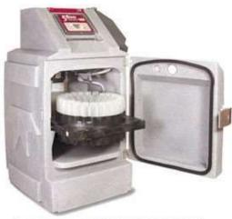
**Isco 5800 Refrigerated Sampler.** A stationary outdoor rated and M certified refrigerated sampler installed in hundreds of WWTP;s and industrial effluents plants throughout Ireland.
